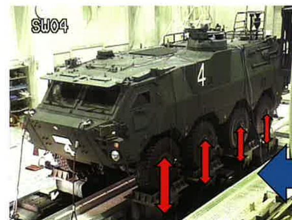
油圧加振機(路面起伏) Hydraulic Actuator (Ground Disturbance)
